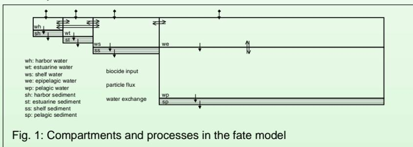
Fig. 1: Compartments and processes in the fate model
